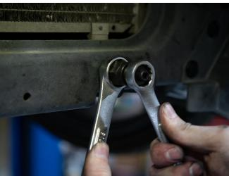
8. With the two 120 degree fittings on the -10 AN oil lines matched up, feed the lines into the gap between the windshield washer reservoir and the front core support, between the two black plastic splash shields, towards the lower oil pan.
