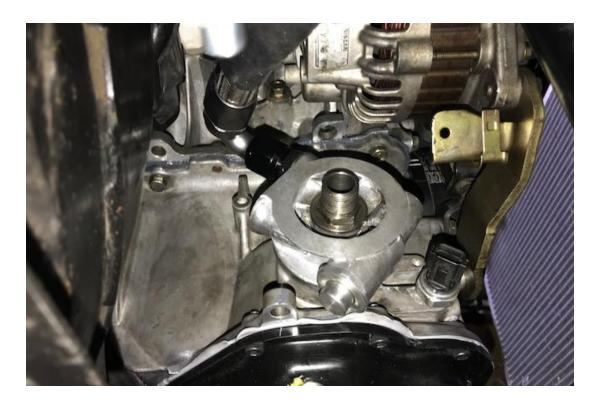
For those who want to keep the stock water-to-oil cooler, you must clock the sandwich plate so the fittings are at about 10 o'clock position, pointing back and up towards the motor mount, making sure to not let the lines make contact with the mount or alternator. Then tighten it down with the provided female to male stud which is a 1 inch (see picture below).
