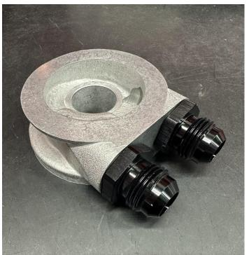
10. Apply a small amount of oil to the o-ring on the back side of the sandwich plate. For those who want to remove the stock water-to-oil cooler, attach the oil sandwich plate to the upper oil pan where the stock engine oil cooler was, and position the fittings so they are at about the 11 o'clock position as pictured below. Tighten it down with the stock male-to-male hollow stud which is a 22mm and will require a deep well socket (see picture below).
