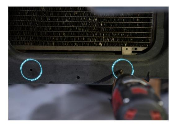
7. Insert the M6 rivnuts and tool and tighten the tool down to crush the rivnut and secure the threads.
