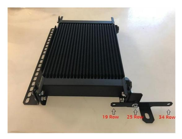
17. Fill up the cooler core all the way with fresh oil to avoid a dry start situation and to help purge all of the air in the lines and cooler faster.
