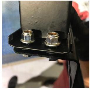
15. Attach the short upper bracket to the cooler core with the two of the supplied 10mm bolts, rubber washers and lock nuts. When all of the brackets have been installed, your core should look something like this:
