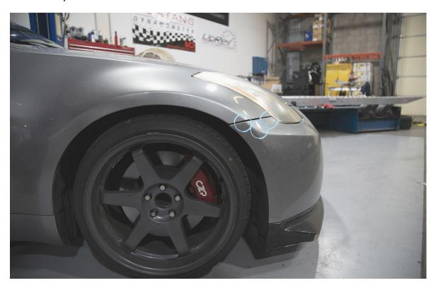
With the wheel turned inwards slightly, you can push the fender liner out of the way slightly and gain access to the two bolts going up into the fender and the one bolt going upward, mounting the bumper bracket to the headlight. All three are 10mm and may require the use of an extension.
