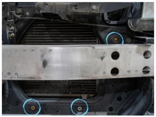
20. Now move the cooler into position and screw the two 10mm bottom mounting bolts into the rivnuts installed in step #7, as well as the 12mm upper bolt that holds the upper brackets.
