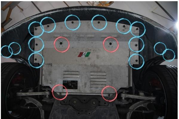
4. Carefully remove the bumper cover. With two people, gently pull the bumper cover forward and away from the body of the car.
