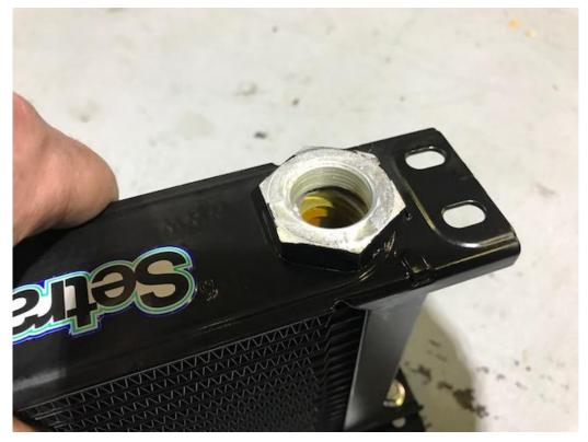
18. Apply a dab of fresh oil to the o-ring seal and thread the remaining two -10 AN to 22mm adapter fittings to the top of the cooler core and tighten them down.
